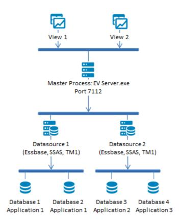
The default behavior of the Performance AL server doesn't use any distribution. All cubes, outlines and data are stored in the memory of the EVServer.exe master process and all client requests are handled by the master process.
