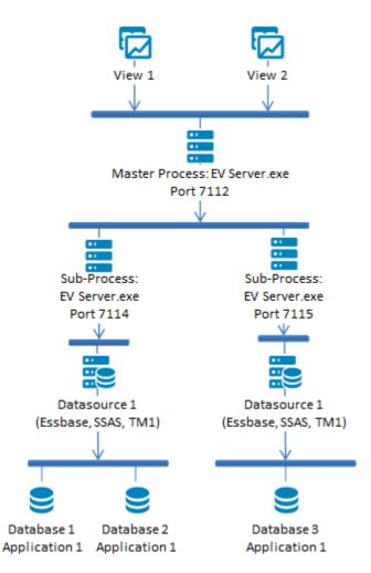
Process distribution can be configured either on Data Sources or on Databases. By default, Databases inherit from their Data Source and apply their settings. However, in some special cases, it can be necessary to remove this inheritance and define a distribution for a specific Database.
